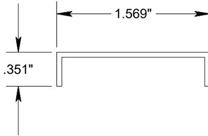
Measurements are approximate - bend to suit/fit at assembly
