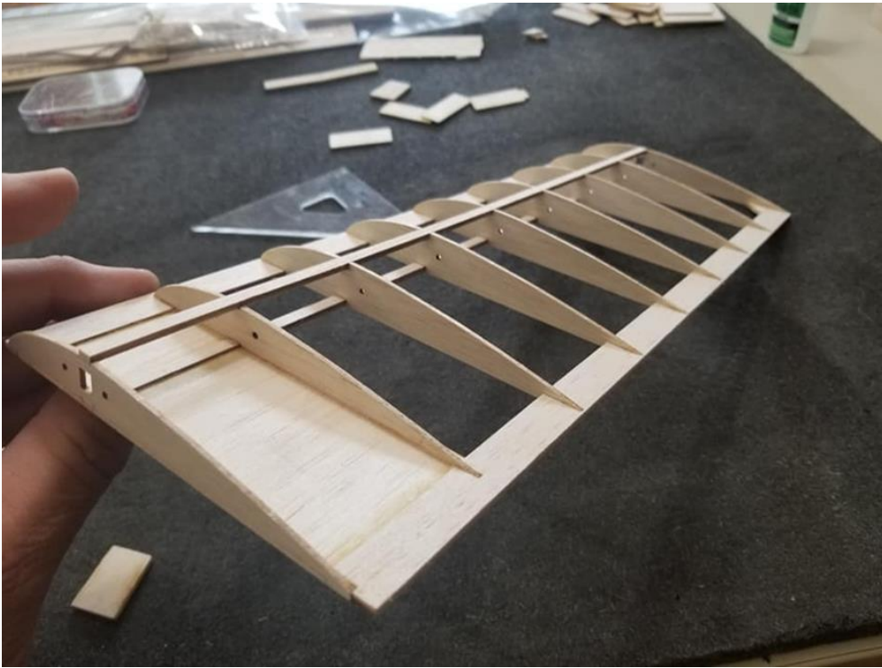
Right side Main Wing Panel with bottom sheeting installed.
