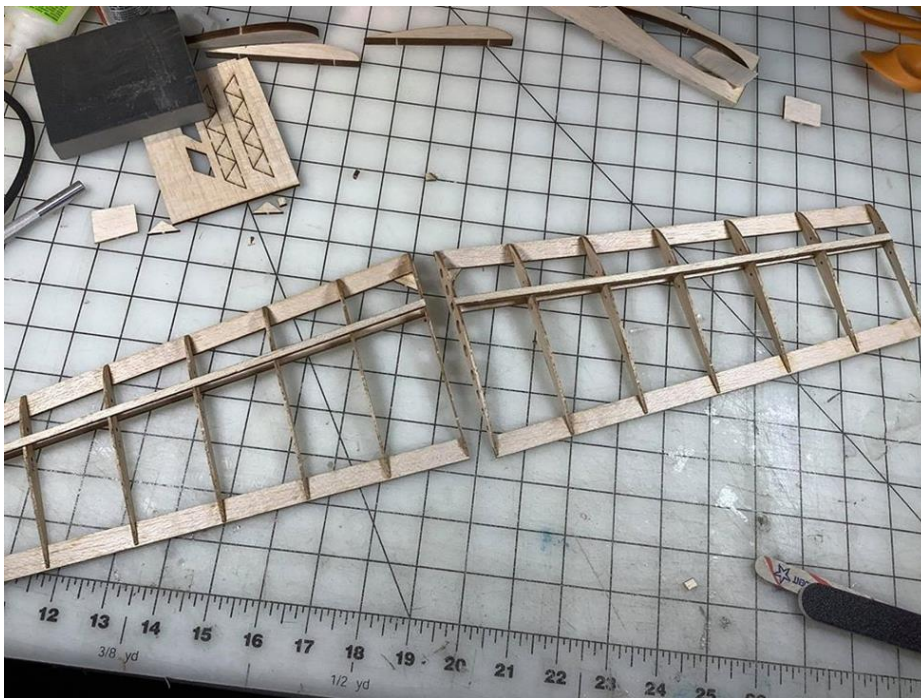
The Outer Wing Panels are assembled the same as the Main Wing Panels. There is a Sweep to the Leading Edge and you can check the squareness at the Root Rib and Trailing Edge. Note the Ribs with Laser cut holes (Root Rib) and the Dihedral tilt.
