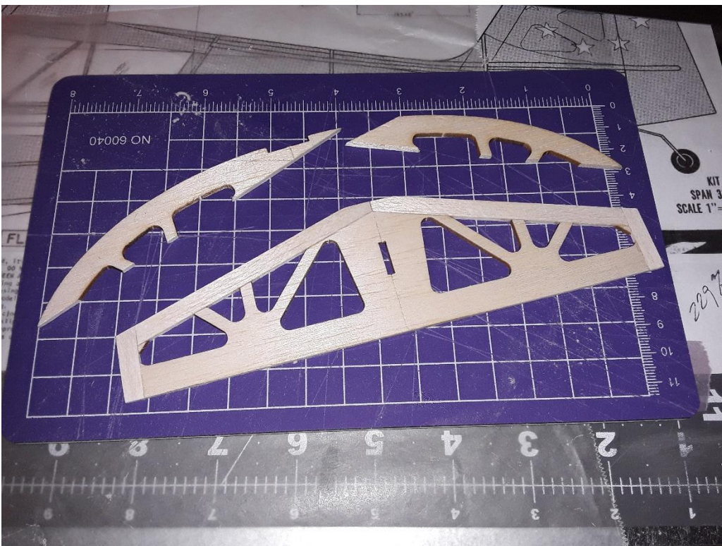
Finished stab ready for final sanding and covering. Trimmed to length, caps added, note grain direction to minimize warps and add stiffness.
