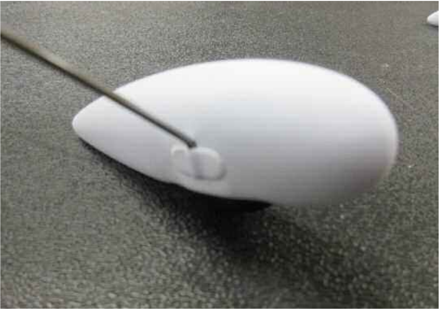
GLUE WIRE GEAR RETAINER WITH MEDIUM CA.
