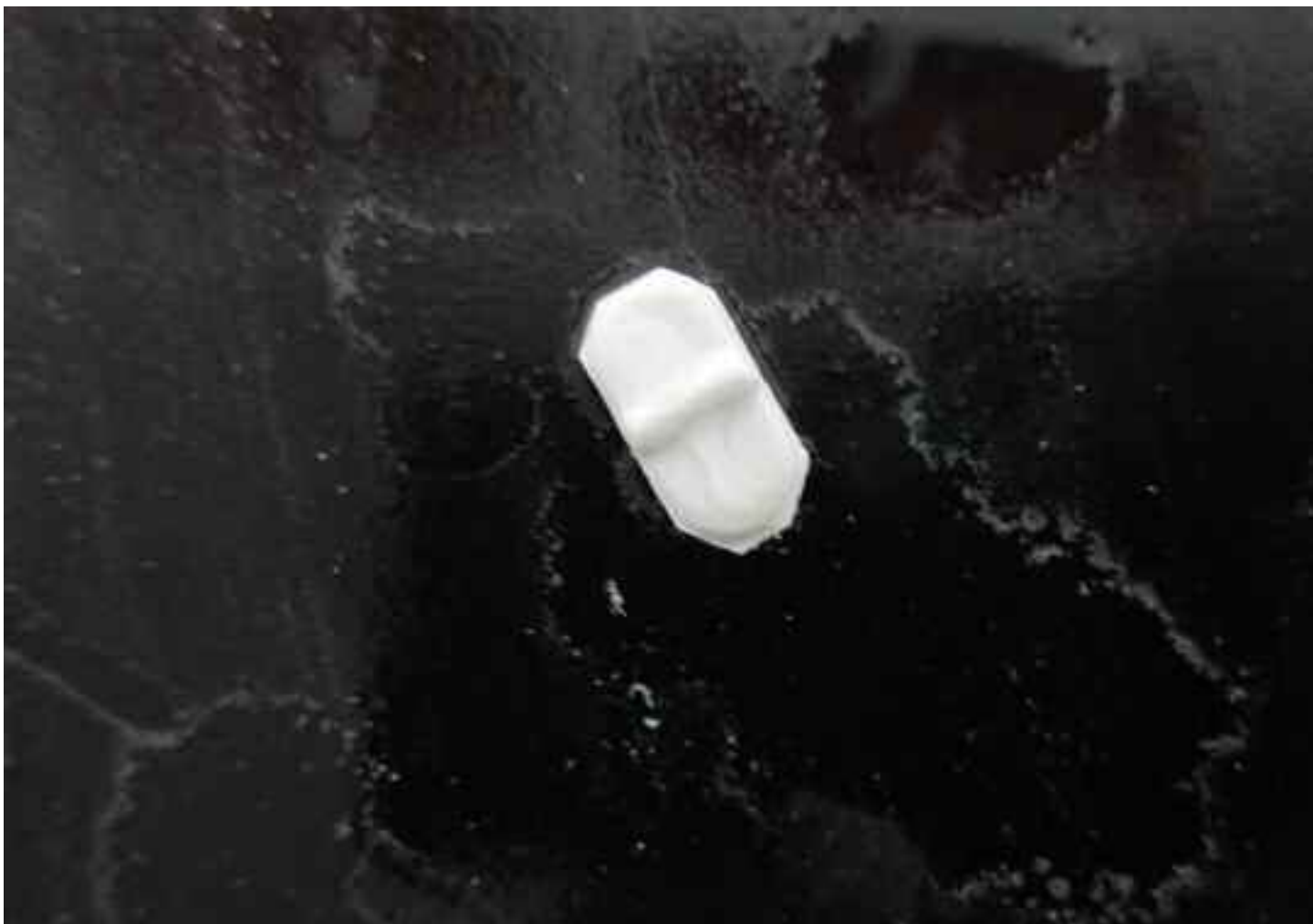
WET SAND WIRE GEAR RETAINERS ON 400 WET/DRY PAPER ATTACHED TO A FLAT SURFACE.
