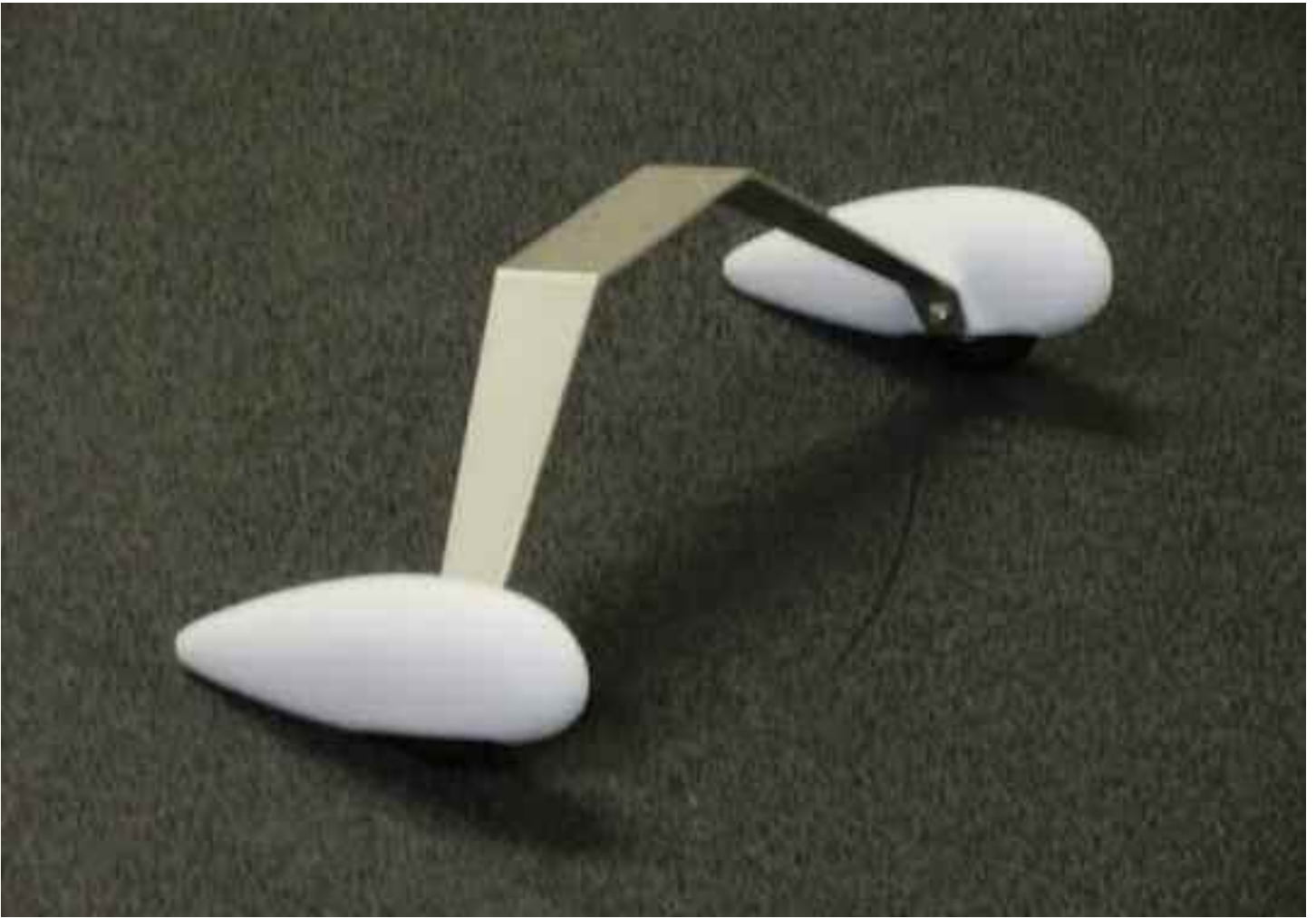
ALUMINUM GEAR MOUNTING
