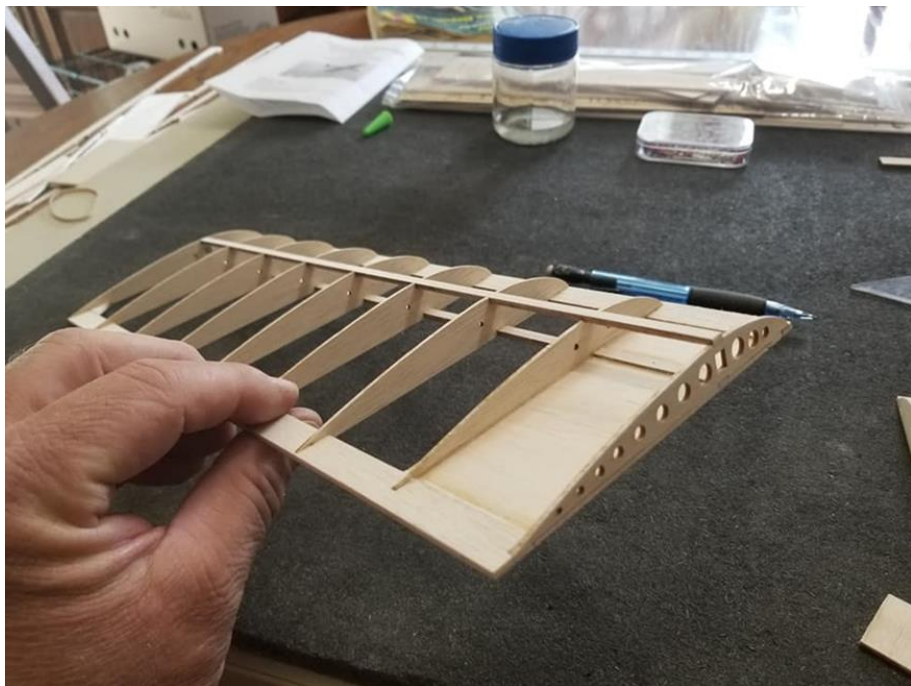
Left side Main Wing Panel with bottom sheeting installed.
